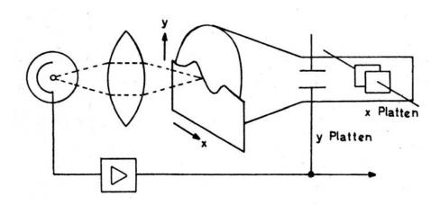
The input to the X-deflection plates determines the position at which the function value has to be determined. The function is implemented as an opaque mask placed in front of the tube screen. A feedback loop will generate an Y-deflection voltage in such a way that the beam will just be on top of the mask, thus following the function.
