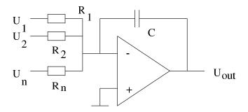
Integration is just as easy as summing – the main difference between a summer and an integrator is that the latter uses a capacitor as its feedback impedance as shown above. The output voltage of the integrator shown above is
