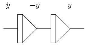
Using a summer with one input the sign of the result can be changed easily:
