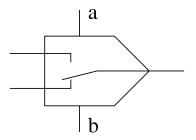
Such a comparator normally has two control inputs a and b. It calculates the sum a+b. If this sum is greater than zero, the relay will be placed in the upper position, otherwise it will be in the lower position.
