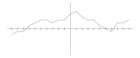
Most implementations have either fixed sampling points (in this case there are normally 21 of these points spaced  $\frac{1}{10}E$  apart where E denotes the machine unit (either 10 V or 100 V)) or variable sampling points.
