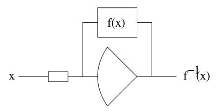
This circuit is normally employed to generate a square root from a square, an exponential function from a logarithmic function, etc.
